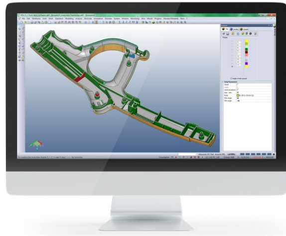
Analysis of draft angles with colour zone representation
